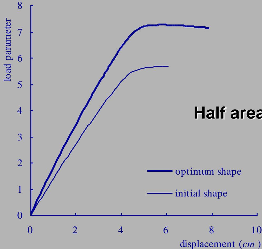
The Load-Displacement Curves at Point a
