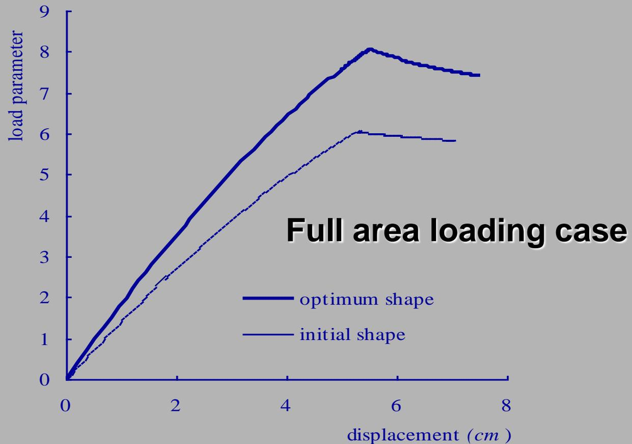
The Load-Displacement Curves at Point a
