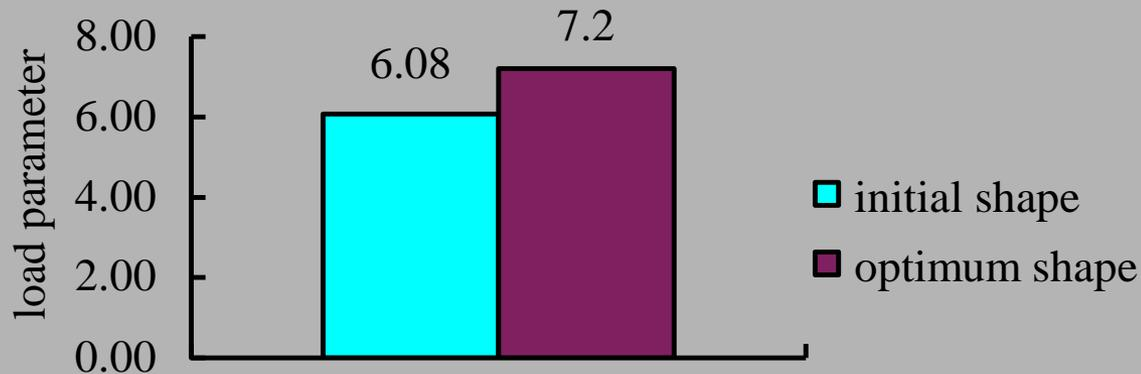
The buckling load parameter increase 18.42%
